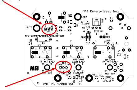
JP2 RIGHT between 2 and 3 (1707) for RF Sense (default), Remove for no RF Sense. Do not place on the left between 1 and 2 (1708) position.
